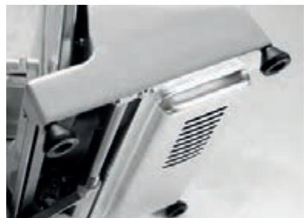
Air cooled engine protected by metal cover
